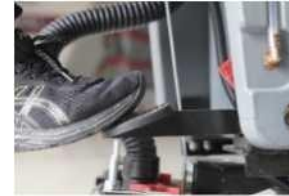
Step 1: step on the pedal pole, put down the washing plate;
