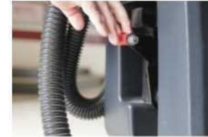
Step 2: through the pull handle, put down the water suction to pick the
