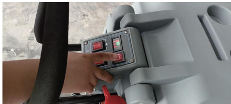
Step 3: Turn on the main power switch, keep driving at a constant speed. start the brush switch button and the water absorption motor switch button;
